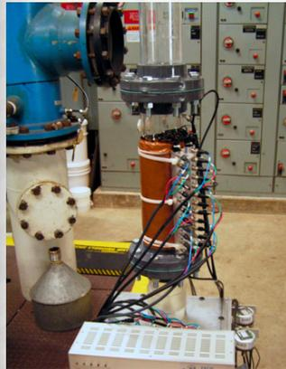
*Measuring solids concentration with electrocapacitance volume tomography.*
