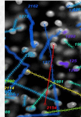
*Tracking of individual particles using high speed particle image velocimetry.*
