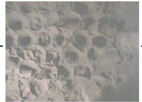
Figure 1. Example of plugged CSC inlet tubesheet [Polk, 2002].
