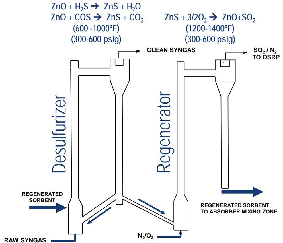
RTI - Eastman High Temperature Desulfurization Process
