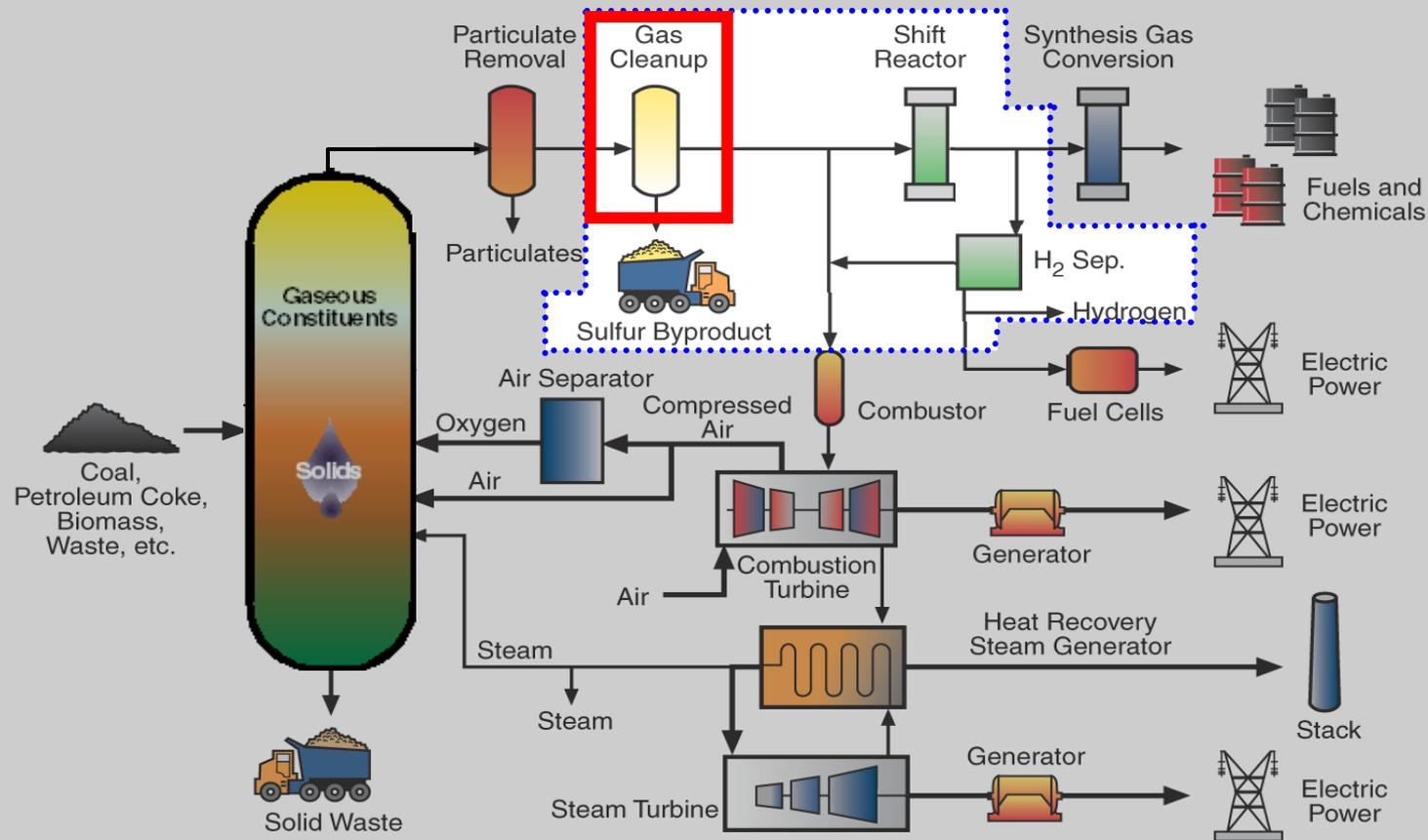
**R&D objective:** Platform of warm syngas cleaning technologies providing improved efficiency, environmental performance, and cost
