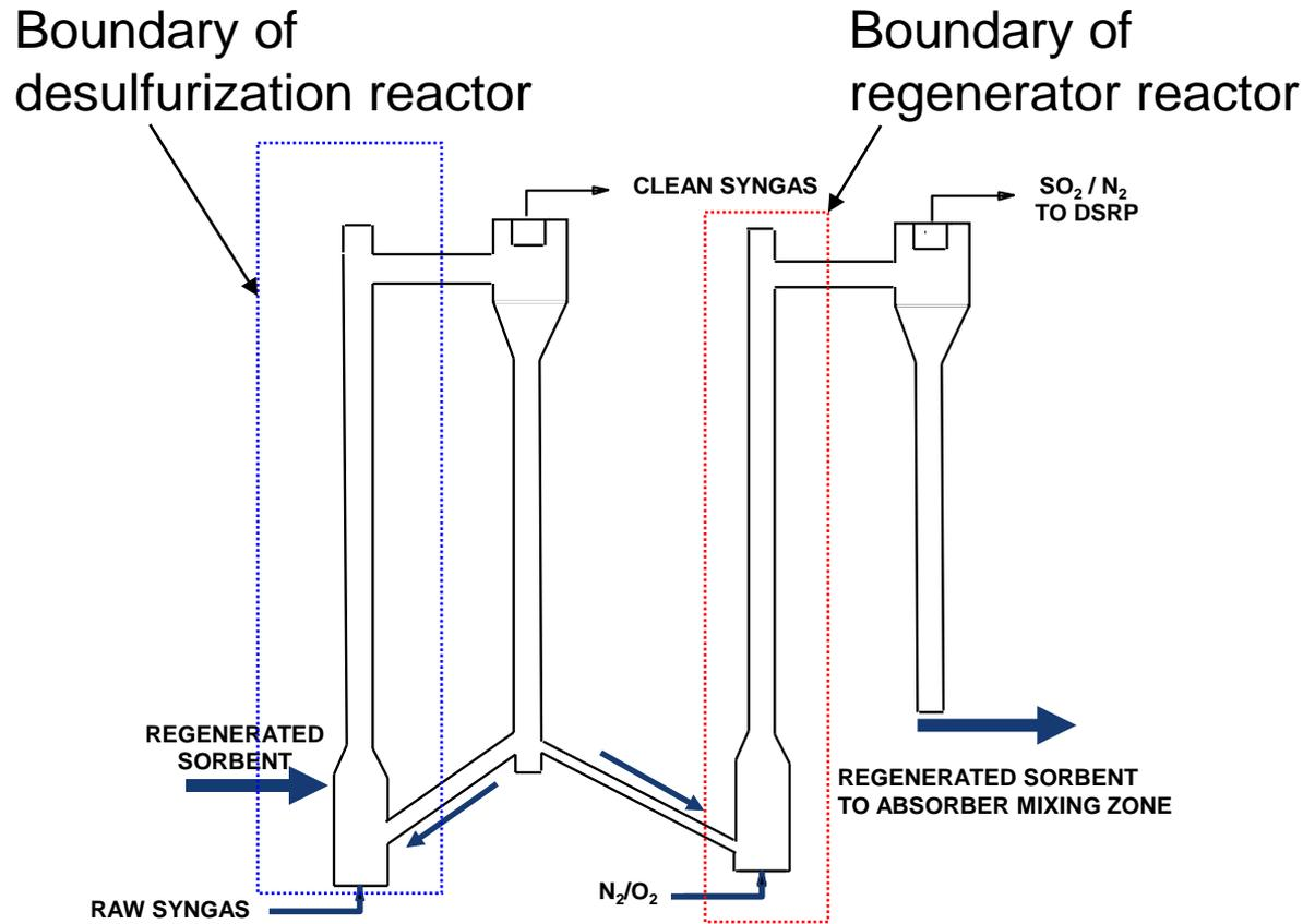
RTI - Eastman High Temperature Desulfurization Process
