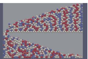
Setup: An inner box with an outlet at the bottom-left is moved vertically in an outer box where particles are discharged
