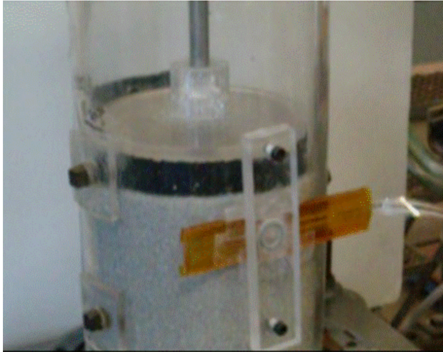
Side view with wall normal stress sensor
