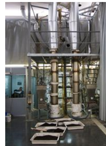
Pilot-scale calcium looping rig (30 kW) at INCAR_CSIC, Oviedo, Spain*
