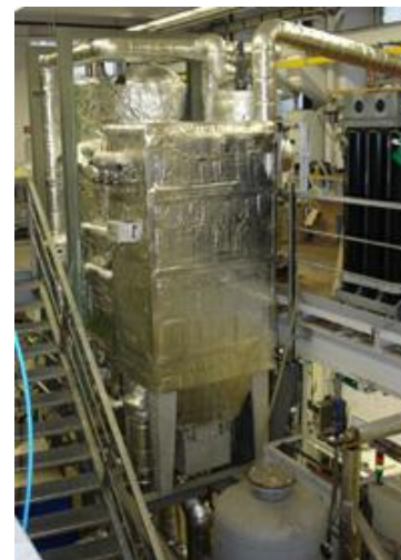
120 kW Chemical Looping test rig (TU, Austria) *
