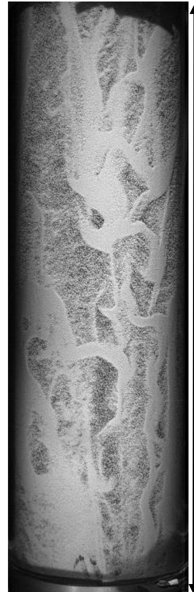
Clusters of 750 \mu\text{m} HDPE in NETL 12" riser
