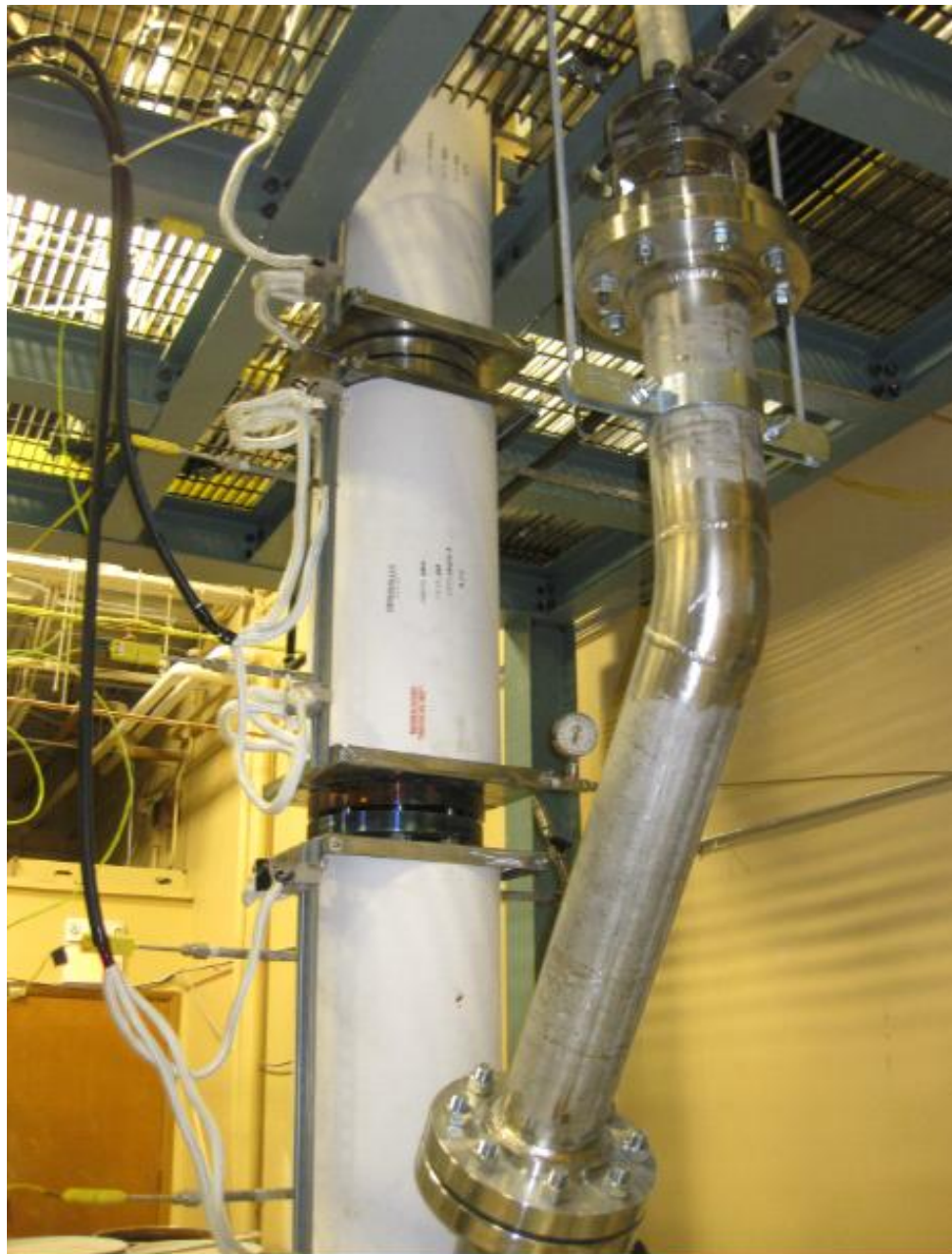
Calcium Looping Sub-pilot Unit for Hydrogen production
