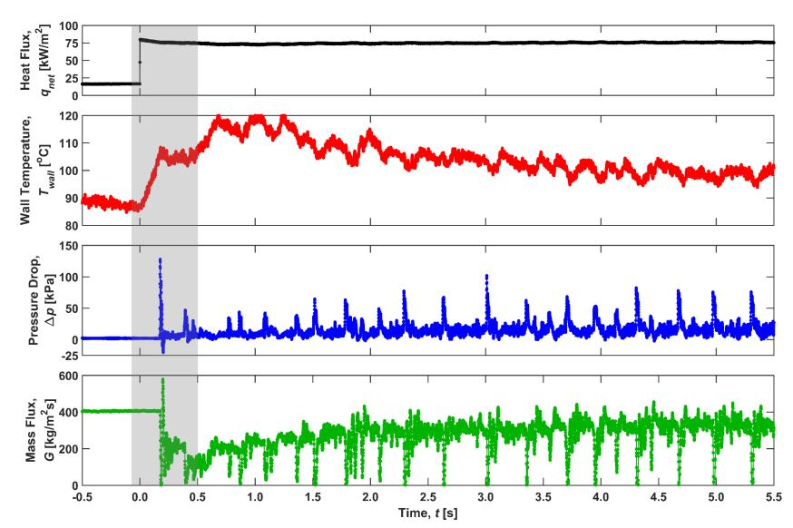
During the transition, the wall temperature overshoots the eventual steady wall temperature by approximately 20 °C
