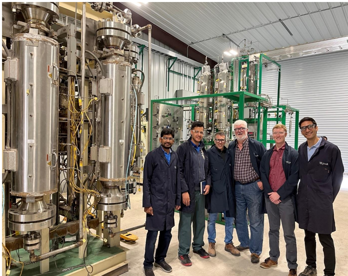
Multiple reactor system holds 100's of kgs of catalyst
