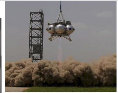
Figure 1. (left) LEM camera views from Apollo 15 landing showing progression of plume-regolith interaction resulting in high-speed particle sheets obscuration. [1](right) Regolith dust cloud formation during Morpheus lander plume impinging on Mars simulant[2].
