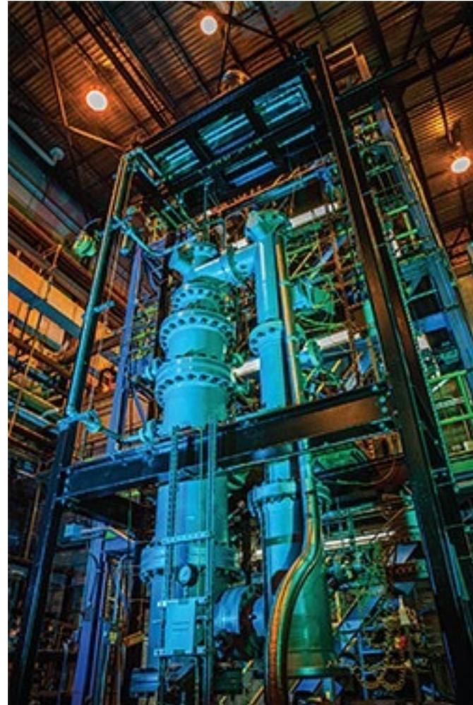
A pilot-scale chemical looping reactor at NETL
