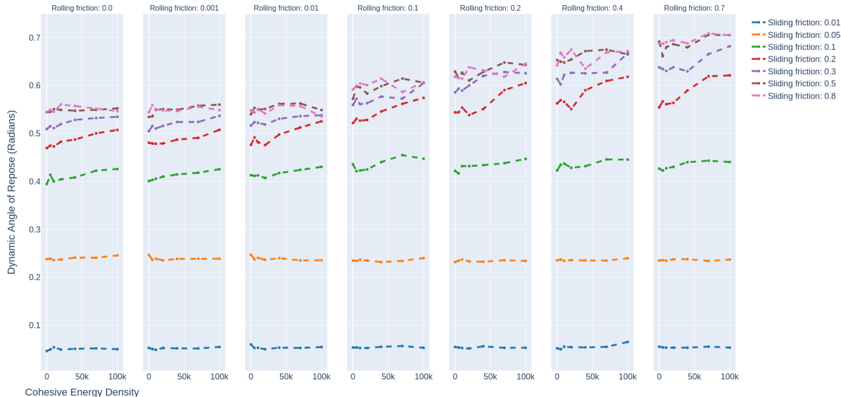
Fig 5: Results of a parameter study looking at the change in dynamic angle of repose due to different values for DEM parameters.
