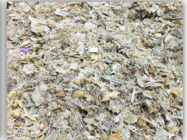
Chipped wind turbine blades
