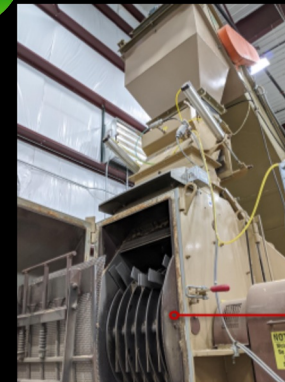
Material jamming in hammer mill grinder
