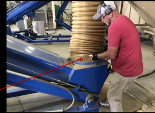
Material clogging in screw conveyor
