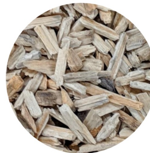
Chipped loblolly pine particles (3-4 mm sieve size)
