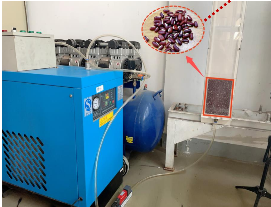
Spouted bed field test bench
