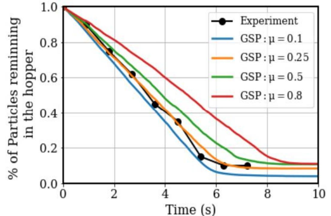
Percentage of particles remaining in the hopper, with different coefficients of friction ( $\mu$ ) used in GSP model.
