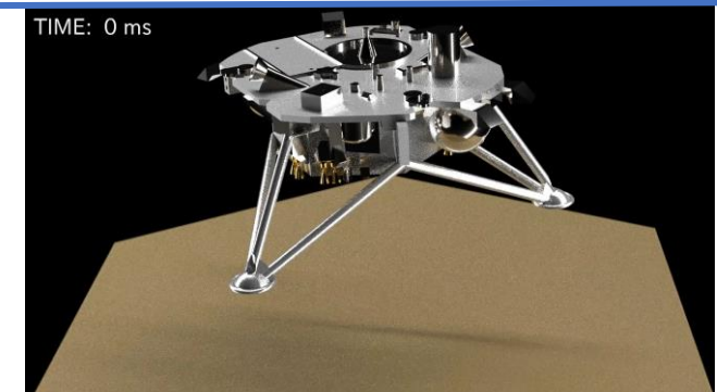
Insight Lander Simulation with 250M Cells on 3k Cores. Courtesy of MSFC/ER42 ESSCA
